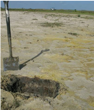
Figure 39. Aerial photograph (above) showing of the exposed sandy dry lake-bed of Lake Alexandrina acid sulfate soil near Paltaloch Station, Narrung area, showing a soil pit (lower left) with black sulfidic material (iron sulfides) overlying sulfuric material with distinct yellow patches comprising mainly the bright yellow mineral, sideronatrite, with a pH ranging between 1.3 to 1.6. (from Fitzpatrick et al. 2008f)
