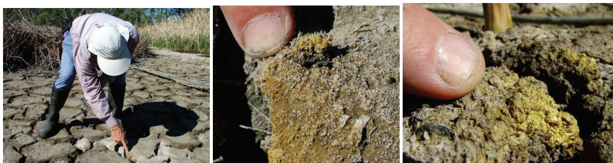
Figure 41 Photograph of Swanport wetland showing: Acid Sulfate Soil with sulfuric material in drained wetlands adjacent to the River Murray (left), which shows extensive cracking and accumulation of scale-like, bright golden yellow crystals of metavoltine ( K_2Na_6Fe^{2+}Fe^{3+}_6(SO_4)_{12}O_2 \cdot 18H_2O ) and white crystals of alunogen ( Al_2(SO_4)_3 \cdot 17H_2O ), which have formed as a result of aqueous, acidic ( pH < 2.5 ), sulfate bearing solutions that have percolated through the soil and attacked layer silicates. These localised solutions were rich in ferrous and ferric iron and also contained leached potassium and sodium. Metavoltine and alunogen are presumed to be the latest minerals to form. The sulfuric material, which also contains natrojarosite, hexahydrate and gypsum developed after drainage when watertable levels had dropped below 40 cm in June 2007 and below 90 cm in November 2007, due to the severe drought conditions, exposing large sections of riverbank and wetlands that once contained high levels of un-oxidized iron sulfide (pyrite). Sulfidic material ( pH > 4 ), which contains un-oxidized pyrite, occurs below the water table. (From Fitzpatrick et al. 2008a).
