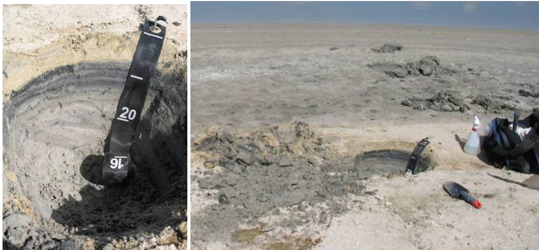
Figure 11. Sulfidic soil at site TB 8 (on the upper shoreline) on the north-west side of the billabong. The dark bands at about 7 – 15 cm are sulfidic material and are likely to acidify on drying.
