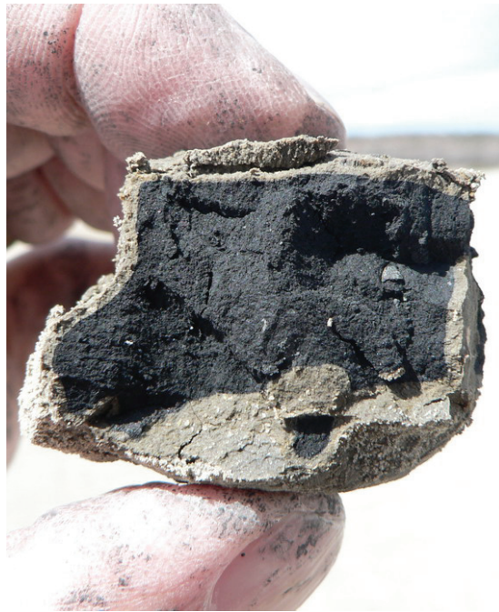
Figure 8. Close-up view of a fractured piece of the dried and hardened surface material at site TB19 showing a brownish, platy surface layer (2 to 10 mm thick) abruptly surrounding the inner, black sulfidic-like material.
