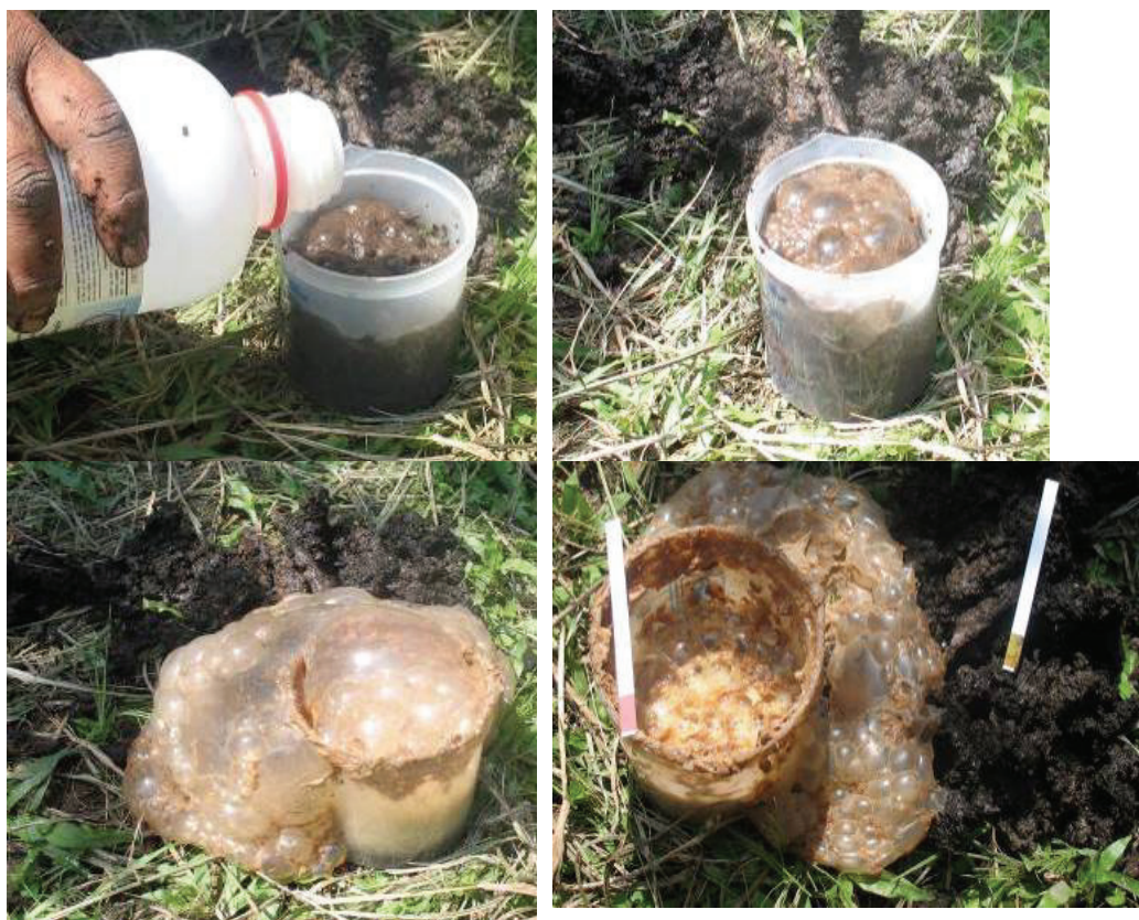
Figure 8: Photographs of the peroxide test in the field used to assess the presence of ASS (sulfidic material). Note the change in colour of the pH test strips indicating the drop in pH. Frothing and fuming are caused by the reaction of peroxide with organic matter and peroxide decomposition catalysed by metal ions. Colour changes to orange and yellow are more indicative of acid formation (from Fitzpatrick et al. 2008c).
