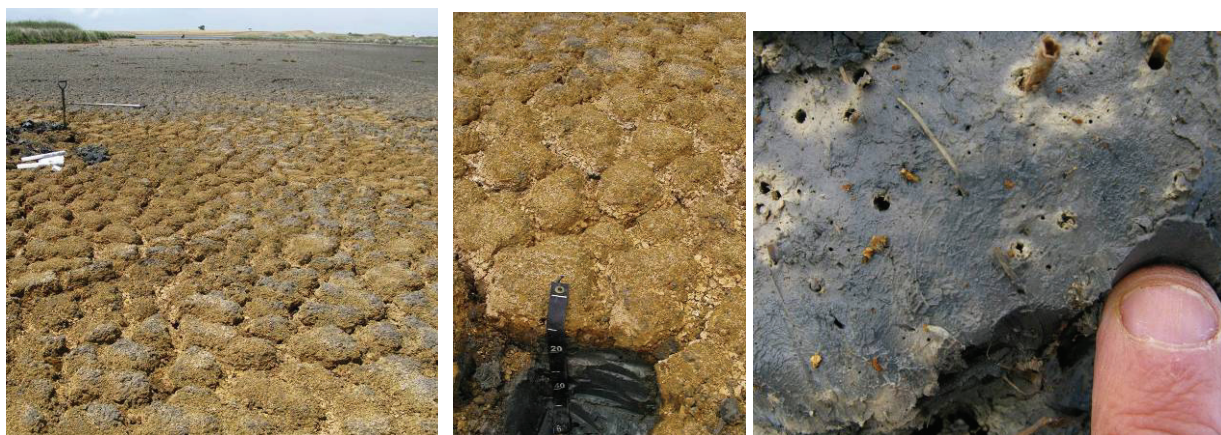
Figure 34. Acid Sulfate Soil in the clayey dry river-bed of the Finnis River, showing a soil pit with black sulfidic material (iron sulfides) at depth (> 60 cm) overlying sulfuric material. Light yellow or straw coloured mottles comprising mainly natrojarosite immediately overlies the sulfidic material between a depth of 30 to 60 cm, which in turn overlies a cracked surface layer (0 to 30 cm) with a pH ranging between 3 to 3.6 comprising mainly the bright orange mineral, schwertmannite. Pale yellow mottles (right hand side) can be seen surrounding old Phragmites root channels in a dark grey matrix. (from Fitzpatrick et al. 2009).
