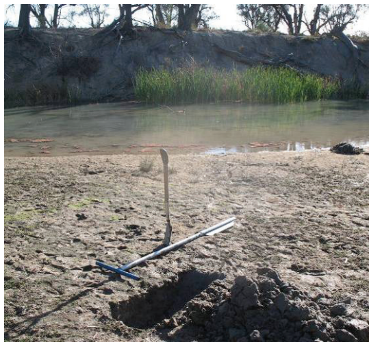
Figure 14. Sulfidic subaqueous soil with thick (0 to 50 cm) soft, sandy, sulfidic material overlying wet clay. Site SC6 was sampled from the stream bed of Salt Creek mid way between the near bank and the reeds on the far side.
