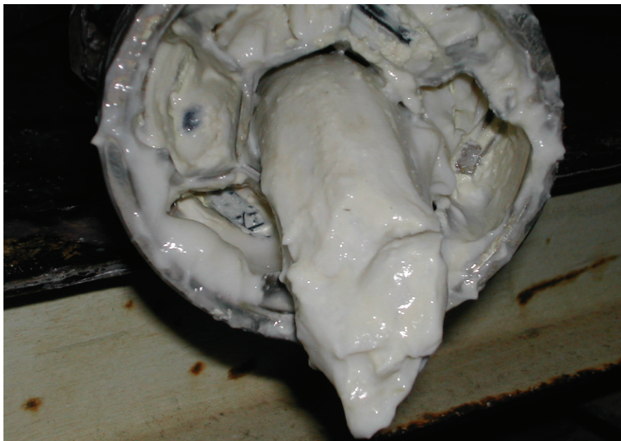
Figure 1. Clogging of pump and impellers by amorphous \text{Al}(\text{OH})_3 (from James-Smith et al 2005).
