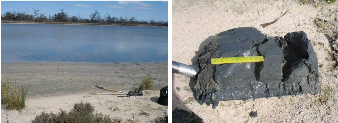
Figure 6. Sulfidic subaqueous soil (wet, soft, sandy sulfidic material overlying wet, heavy clay sulfidic material). This site, Site TB7, was sampled in water 20 cm deep.
