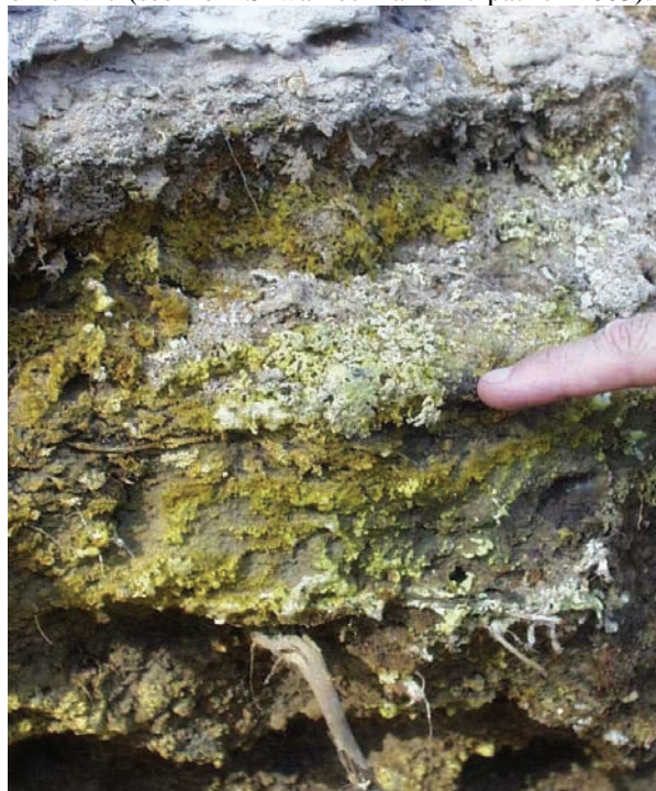
Figure 37 A highly saline sulfuric material (pH 2.5-3.5) exposed along upper Dairy Creek, showing green crystals of sideronatrite ( \text{Na}_2\text{Fe}(\text{SO}_4)_2 \cdot \text{OH} \cdot \text{H}_2\text{O} ) formed in sandy layers and derived from the oxidation and dissolution of the pyrite framboids. Profile N25 (see Figure 28).
